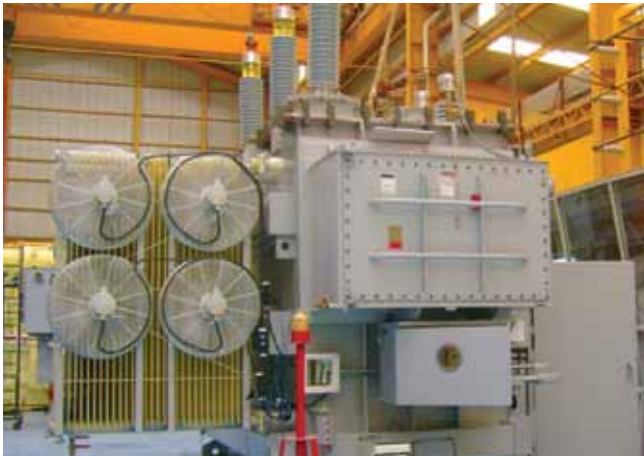
LOWER COLORADO RIVER AUTHORITY Austin, TX 18/24/33 MVA – 138kV
