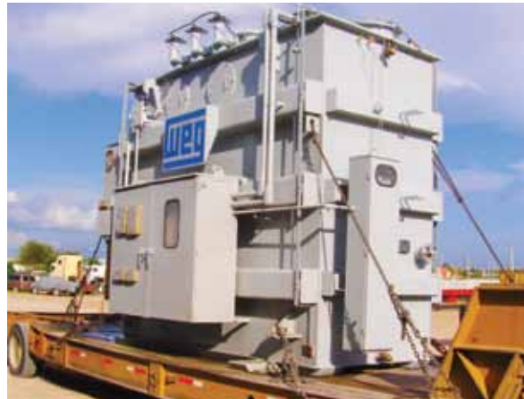
CITY OF EDMOND Edmond, OK 12/16/20 MVA – 138kV
