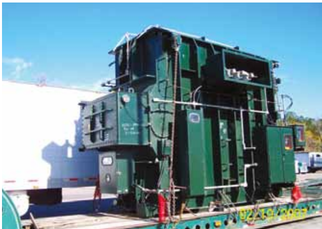
CITY OF TALLAHASSEE Tallahassee, FL 50 MVA – 115kV
